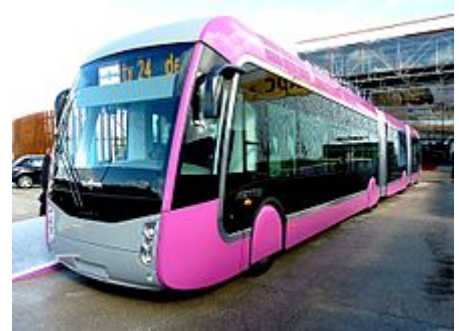
The pink bus rapid transit of Metz uses a diesel-electric hybrid driving system, developed by Belgian Van Hool manufacturer. [55]
