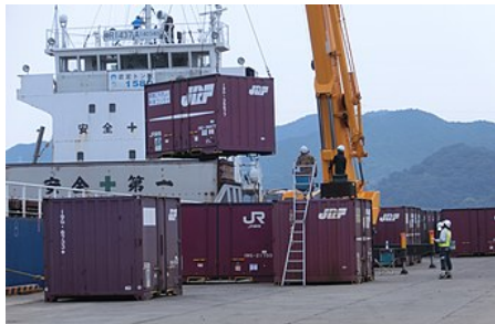
12-foot (3.66 m) the 19D-type container used by JR Freight in Japan
