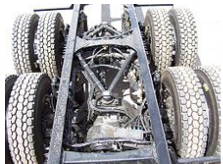
A truck rear suspension and drive axles overview
