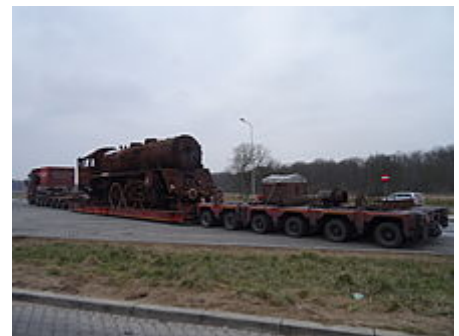
Steam locomotive on hydraulic modular trailer
