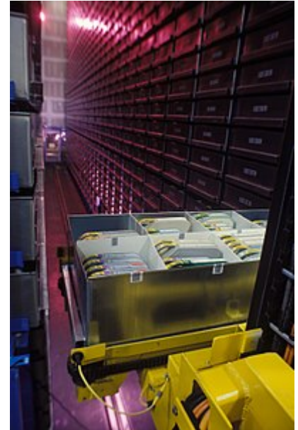
Automated storage and retrieval system used by the U.S. military, also used by business in conjunction with manual picking.
