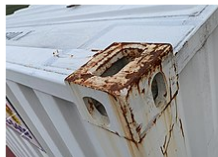
The standard casting that is located on each of the eight corners of a container. The twistlocks fit through the larger oval hole on the bottom castings. Top casting ovals hold twistlock fittings used to secure another container on top.
