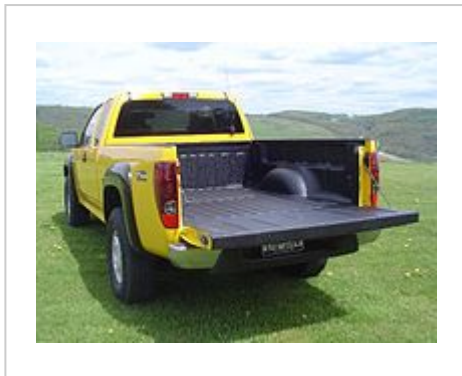
Flat sided pickup truck showing wheel well intrusion into bed.
