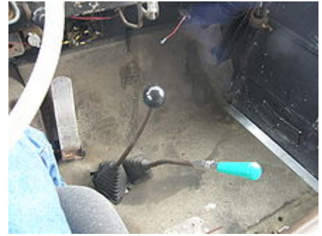
Traditional manual transmissions have 4-5 ratios on main shift and 3-4 on the auxiliary: pictured is a 5×3 with five main ratios and three auxiliaries
