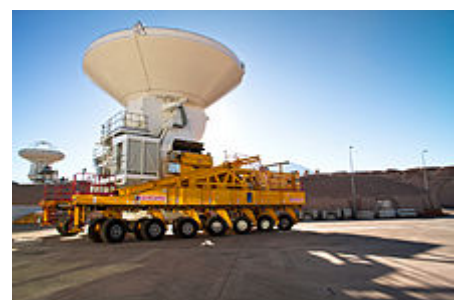
ALMA antenna transporters are 20 m ( 65\frac{2}{3} ft) long, 10 m ( 32\frac{7}{9} ft) wide, weigh 130 t (127.9 long tons; 143.3 short tons) and drive on 28 tires. [20]
