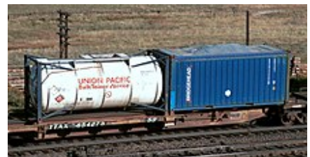
A spine car with a 20 ft tank container and an open-top 20 ft container with canvas cover
