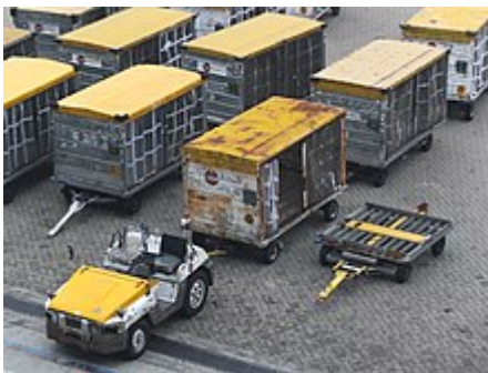
A single trailer for an aircraft cargo unit load device, next to a group of trailers for loose luggage.
