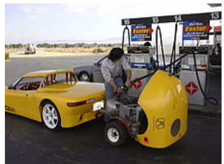
ACP Backtracking genset trailer
