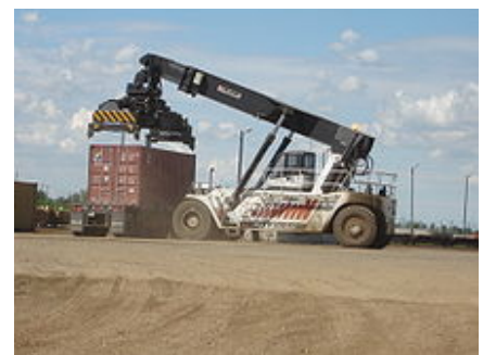
A cargo container being transferred from a rail car to a flat-bed truck, lifted by a reach stacker
