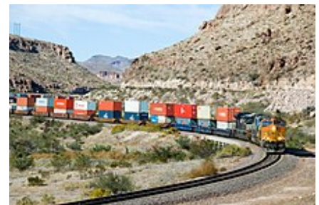
Train in Arizona, with 20-, 40- and-53 foot containers double stacked in well cars
