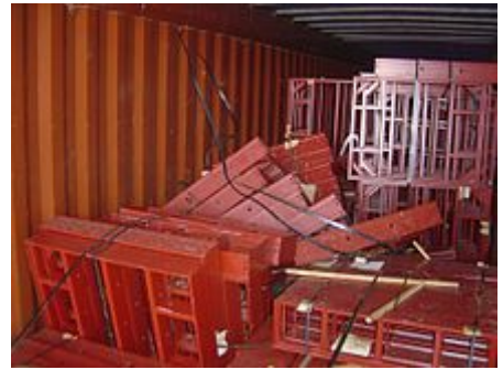
Cargo damage because of improperly secured cargo
