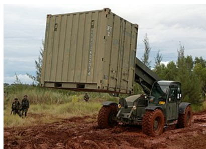
U.S. Navy moving a Bicon box. Note the forklift pockets only in the sides, not at the ends.
