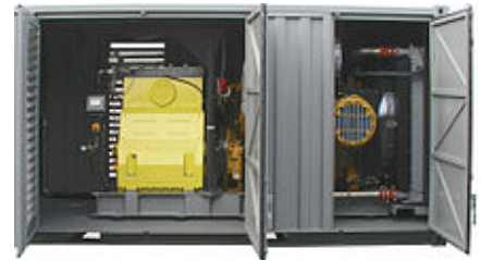
Hammelmann diesel unit [119] built into container
