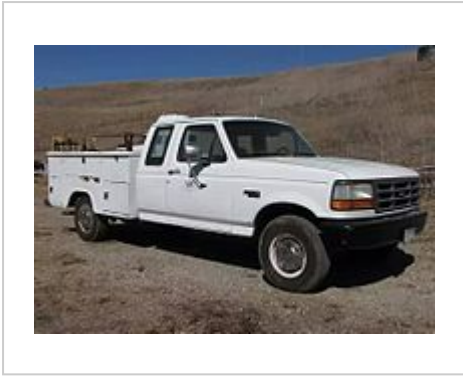
Ford F-250, which was originally sold as a chassis cab, fitted with an aftermarket utility bed.
