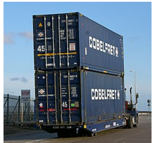
Two 45-foot 'High-cube' containers on a roll-on/roll-off (RoRo) tractor. The text in the yellow arrow on the top unit indicates its extra 2.50 metre ( 8'2\frac{1}{2}" ) width.
