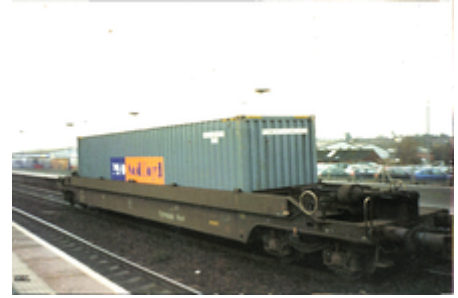
P&O Nedlloyd intermodal container in a tiphook intermodal freight well wagon at Banbury station, England , (2001)
