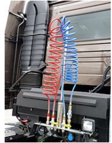
A pair of semi-trailer "Suzies" at the back of an Australian prime mover, red line for emergency/supply and blue for control
