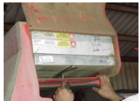
Truck cab filter housing using a contiguous series of pre-, HEPA, and charcoal panel filters
