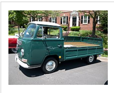
Volkswagen Type 2 with single cab over and a dropside bed with the left panel folded down.
