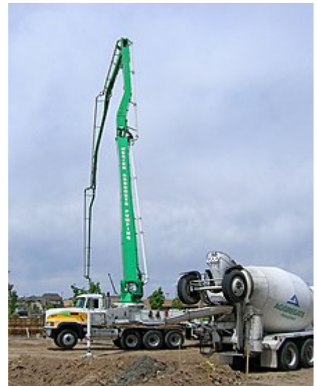
The back of the concrete mixer truck carries a 'booster axle', which can be lowered to extend the wheelbase of a fully loaded truck to comply with regulations. [3]
