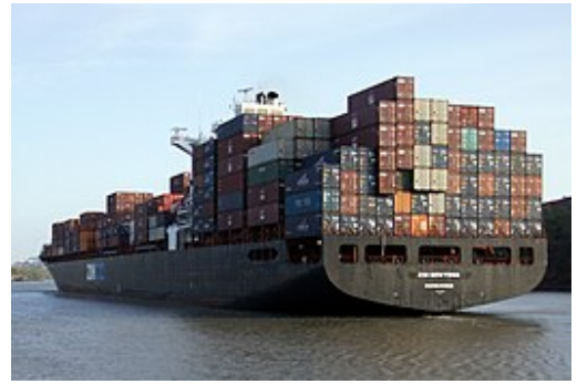
Forty-five-foot containers can be seen sticking out 2.5 feet (0.76 m), as part of the forty foot container stacks at the back of this ship.
