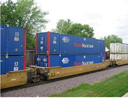
An articulated double-stack well car owned by the TTX Company . The 53 ft (16.15 m) capacity car is a Gunderson Maxi-IV .
