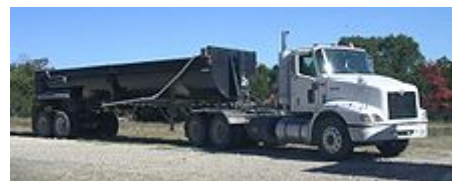
Tractor with an end-dump trailer
