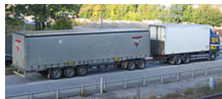
A truck with a swap body pulling a trailer using a dolly ; the overall length is 25.25 m (83 ft)
