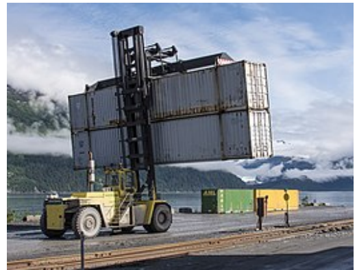
Container "Toplifter" forklift moving two empty 53-foot boxes by their 40-foot posts
