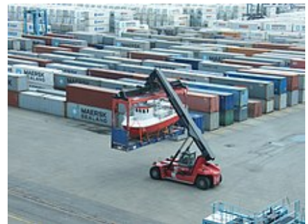
A flat-rack container loaded with a small vessel loaded by a reach stacker.
