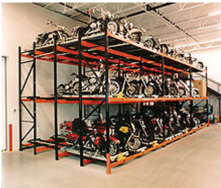
Push-back rack for motorcycles, a LIFO rack system for storage
