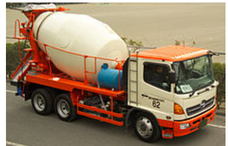
A Japanese concrete mixer
