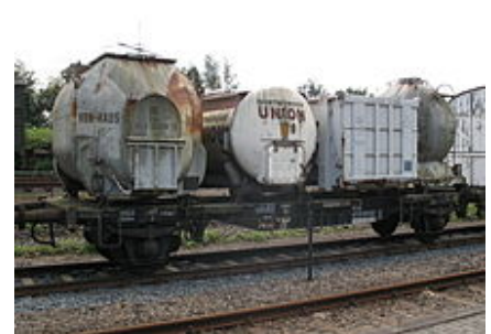
Freight car in railway museum Bochum-Dahlhausen , showing four different UIC-590 pa-containers
