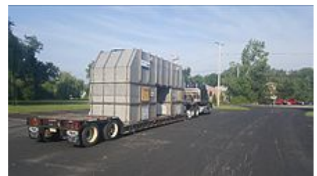
Loading of a thermal oxidizer at the point of origin en route to a manufacturing plant
