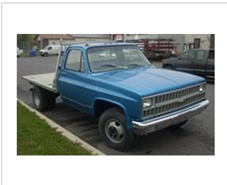
Dually Chevrolet flatbed with dual wheels on the rear axle for improved towing.
