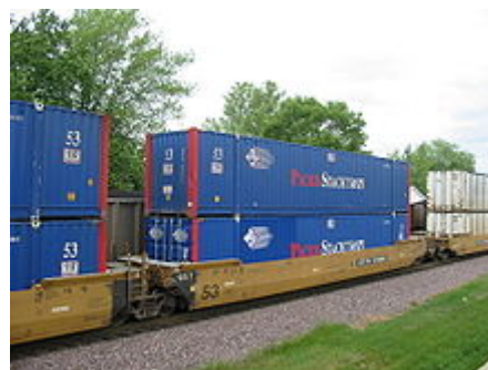
A portion of a "double stack" container train operated by Union Pacific Railroad ; the containers are owned by Pacer Stacktrain , the cars by TTX .
