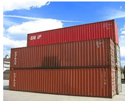
Forty foot (12.2 m) containers make up 70% of the world's container volume, which is measured in TEUs [7]
