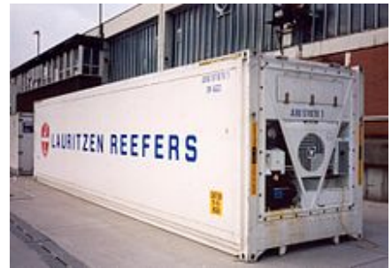
Forty foot High-Cube actively refrigerated container – refrigerating equipment visible on the front end.
