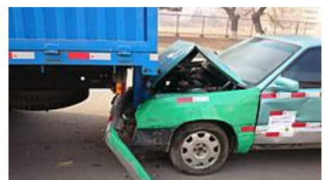
Crash test of an underride guard at 30–40 km/h (19–25 mph); the truck platform at head height has been prevented from slicing through the windshield
