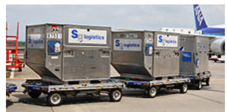
Unit loads for transportation of luggage at the airport. In this case, the unit load has a protective function.
