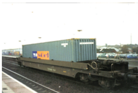
A P&O Nedlloyd intermodal container in a Tiphook well wagon at Banbury station in the UK in 2001
