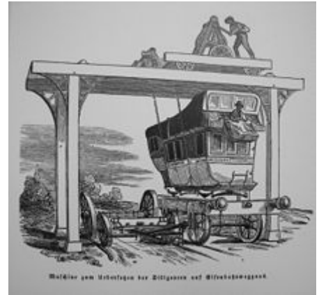
A stagecoach transferred to a railroad car with a simple gantry crane , an example of early intermodal freight transport by the French Mail, 1844. The drawing is exhibited in Deutsches Museum Verkehrszentrum , Munich, Germany.
