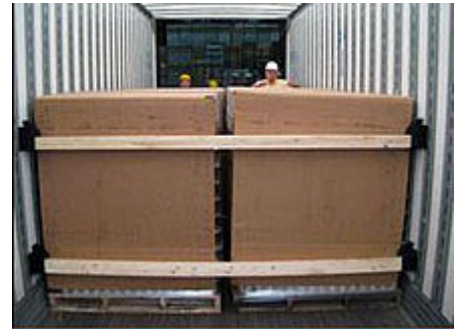
Blocking and Bracing with timber
